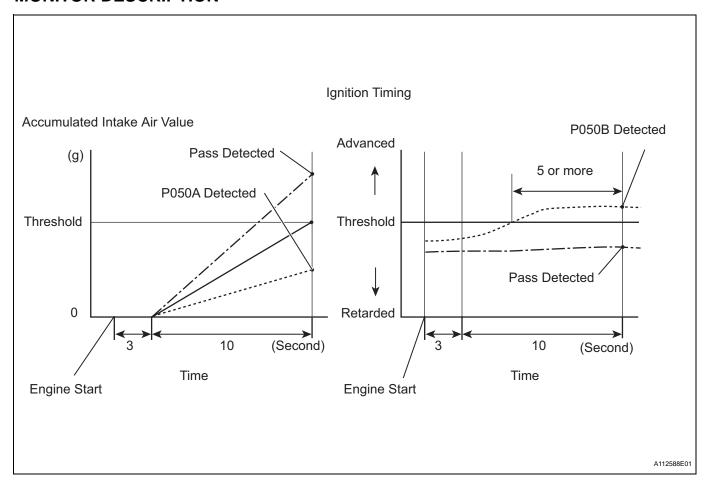
The ECM monitors the intake air amount during idling and the ignition timing.
